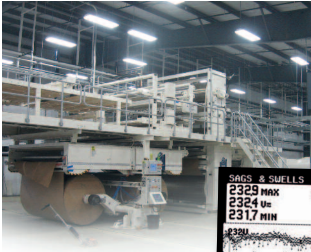
RIGHT: A POWER QUALITY METER READING TAKEN BEFORE THE WPS GLOBAL SYSTEM IS INSTALLED. THE VOLTAGE AND AMPERAGE LEVELS DEMONSTRATE DIRTY POWER.
